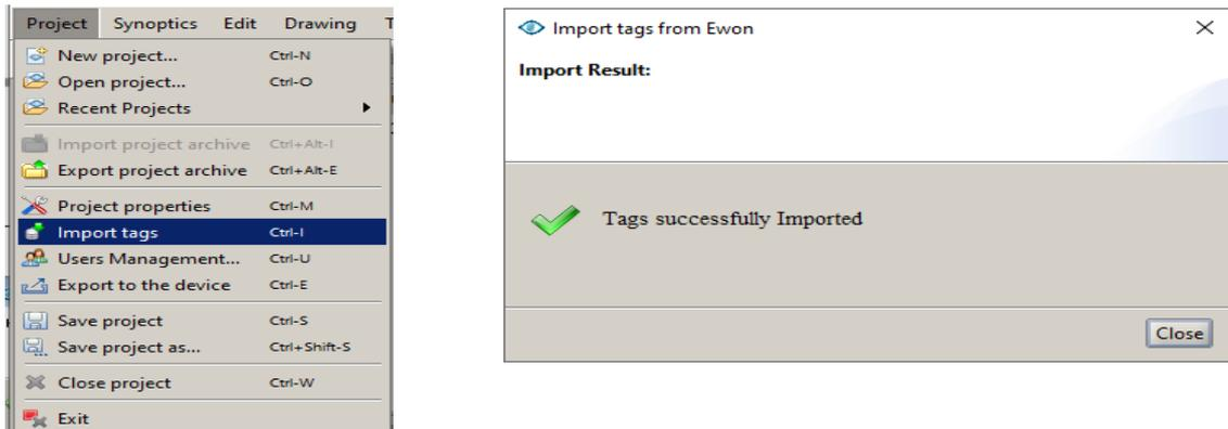
If the HTTP transfer has been done successfully, the above message should appear. The Tags should then be imported from the Ewon device to the viewON project.
