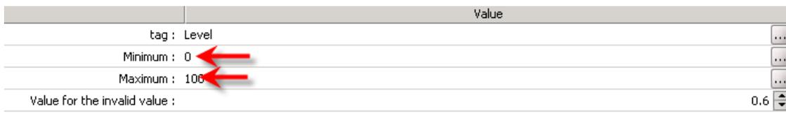
When the value of the linked Tag is less than 0 and more than 100, then the object will 60% opaque (**Invalid value**)
