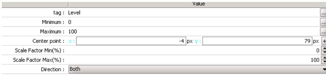
For instance, if you insert 200 (in the **Scale Factor Max** field), then the object will be double-sized.
