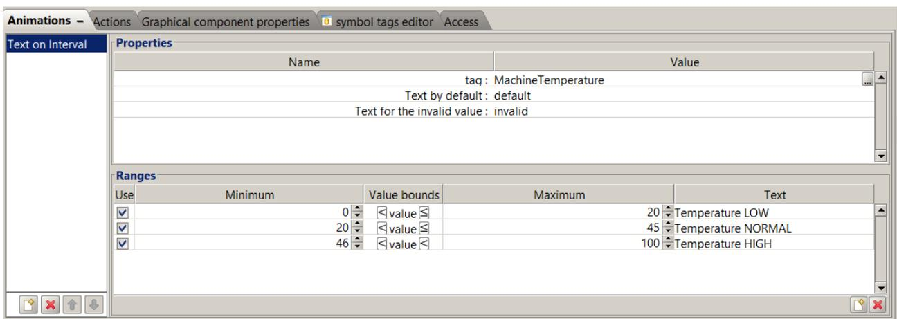
In our example the text 'Temperature LOW' will be displayed if the temperature is between 0 and 20 (included).
