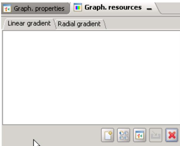
As you can see, both tabs are empty. Let us use the **Linear gradient**, to add a gradient. Click on the **"New"** button, a black gradient called "linear0" will appear. You will work on it to create the color and effect you would like to have.
