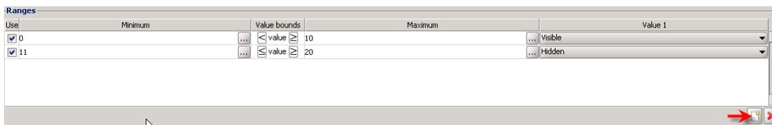
You have to enter values in the **Ranges** section to be able to make your object visible or hidden for different value bounds. For instance, according to the value (visible or hidden) that you have introduced for each range, the object will be visible or not.
