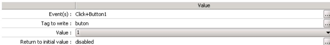
The **Return to initial value** option allows to force viewON to write back automatically the initial value of the Tag after a certain time.
