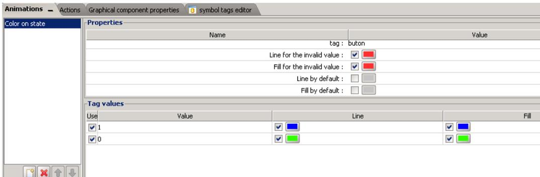
The above picture shows that when the Tag value is 1, then the object will become blue. On the other hand, when the Tag value is 0, then the object will become green. The invalid value colors will be used when the value of the Tag is neither 0 nor 1.
