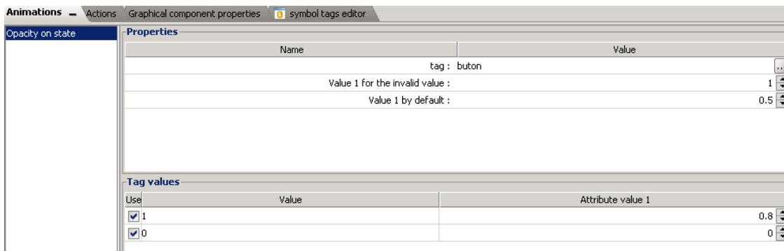
In the **Properties** section, choose the value for the invalid and the default value. In both cases, the maximum is 1. The example in the above picture shows that if the value of a Tag is 1, the object will be 80% opaque. On the other hand, when the value of a Tag is 0, the object becomes invisible.
