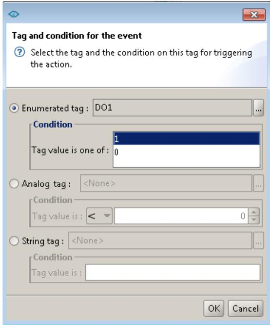
You can then use for your condition an enumerated Tag (Boolean, Alarm Status, Alarm Type), an analog Tag, or a string Tag.
