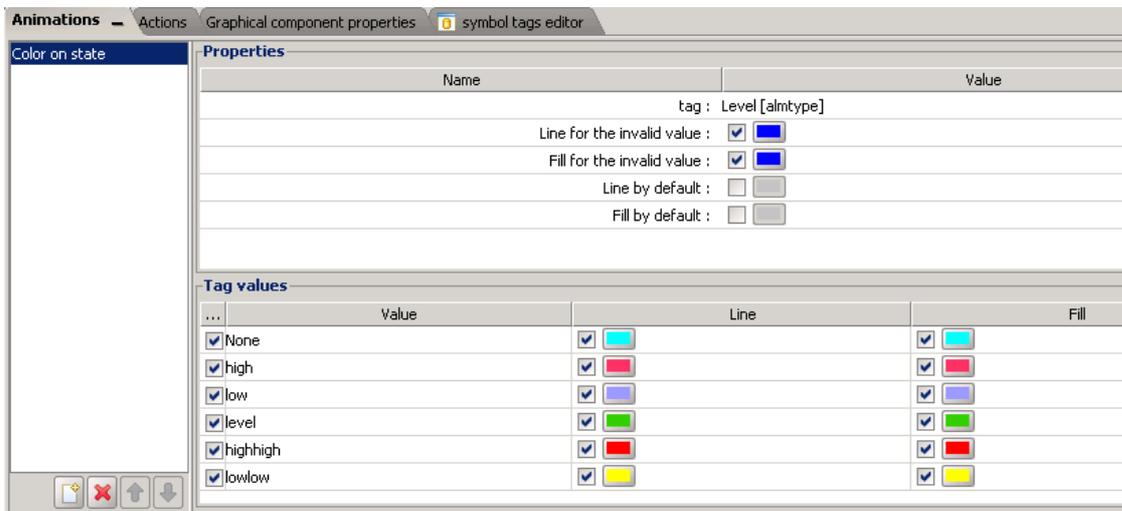
In our example, if the alarm state of the Tag is high (warning), the object turns pink. If the alarm state of the Tag is high high (alert), then, the object turns red, meaning that you need to make an action. The same occurs with the low (warning) and low low alarm state (alert).
