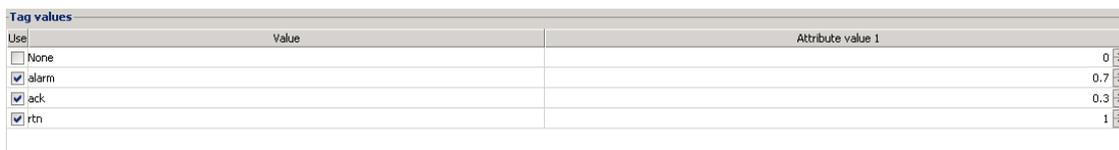
If you chose to apply the opacity to the alarm state, then you will have to apply a value for each status of the alarm (ALM/RTN/ACK). Do not forget that you can also uncheck the statuses and keep only one of them or none.
