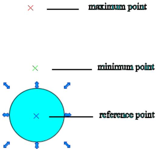
Finally, choose the direction you want the object to move (horizontal/vertical/both). If the minimum point of the Tag is 0 and the maximum is 100, then the object (the reference point) will move linearly from the minimum to the maximum. But if the value is under 0 or above 100, then the object will return to its initial position.
